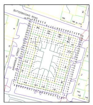
Drilling work was carried out from the streets surrounding the blocks using versatile Casagrande C6 rotary percussive drilling rigs with multi-angling kinematics however for Block 1, at our suggestion, it was agreed to complete a large proportion of the drilling from the rear courtyard.
